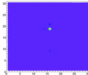
**Fig. 7.** Response of the 2D detector array to a  $^{90}\text{Sr}$  beta source.
