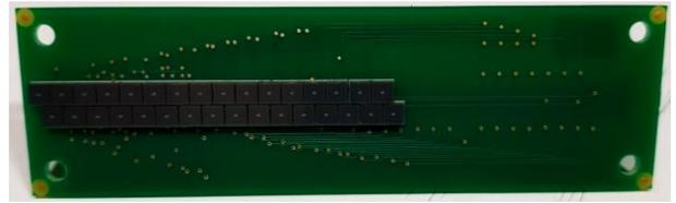
**Fig. 4.** A photograph showing a prototype printed circuit board with 32 Hamamatsu SiPMs.
