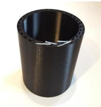
**Fig. 8.** A photograph showing the 3D printed cylindrical scintillating fibre holding structure with 4 exposed fibres.
