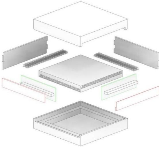
**Fig. 2.** A CAD rendering showing the final 3D printed detector holding structure, enclosed to reduce light interference and improve circuit board support. The SiPM sensor arrays are in green outline colour. Scintillating fibres are inserted in scintillator holding structure in the centre of the image.
