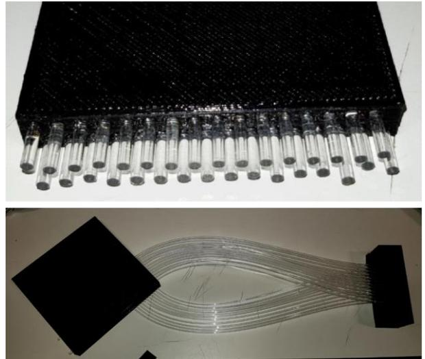
**Fig. 5.** Top: Linear array of 32 fibres in two layers, Bottom: readout of a 3D-printed two-dimensional array, partially filled with scintillating fibres. The operation of the square array was verified with cosmic-ray muons and with a  $^{90}\text{Sr}$  beta source. The histogram in Fig 6 shows cosmic-ray data collected over several hours. It clearly shows the points of intersection of the scintillating fibre matrix, due to coincident events occurring in both layers of fibres.
