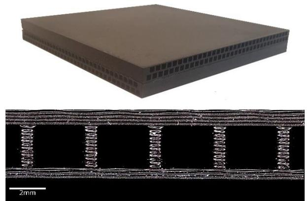
**Fig. 1.** Top: A photograph showing the 3D printed scintillating fibre holding structure, and Bottom: A microscope image showing the channels/openings through the 3D printed structure (scale bar for reference is 2mm).
