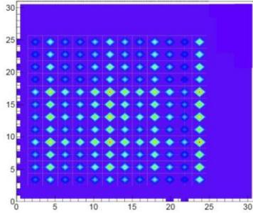
**Fig. 6.** A 2D histogram of hits from cosmic ray muons on the set up shown in Fig 5. The points at which the fibres cross can easily be seen, showing the expected regular square grid and 144 crossover points.
