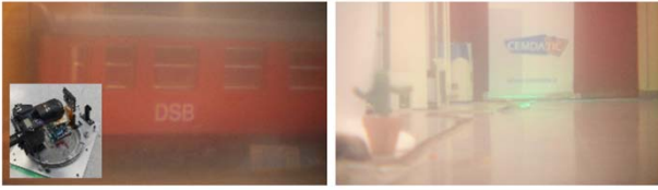
Fig. 4. Two full frame images showing the lens performance when used in front of a digital camera (inset). Changing only the ALL lens electrical addressing images could be captured at 0.5 and 12 m distance to the camera. The camera depth of field was deliberately minimised to highlight the ALL lens effect, by opening the diaphragm (setting the f-number to 3.2)
