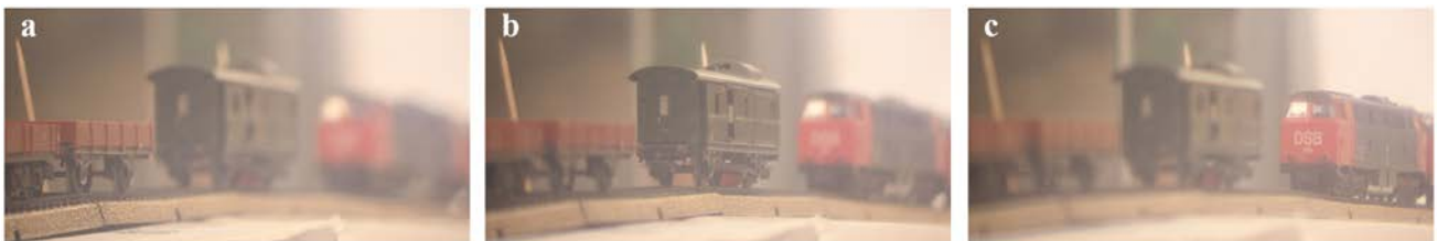
Fig. 5. Details from images using three successive lens settings. a: ALL lens inactive –no topological charge ( N_T=0 ); b: Minimal ALL lens focusing ( -0.15 dioptres \sim N_T=-1 ); c: Twice minimal ALL lens focusing ( -0.30 dioptres \sim N_T=-2 ). Notice how the image quality isn't compromised at all by the ALL lensing, while the focal plan is shifted.
