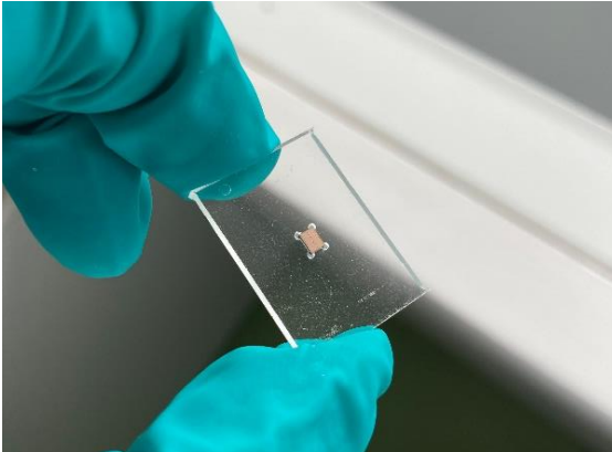
Fig. 4: Silicon photonic sensor chip with packaged with microfluidic.
