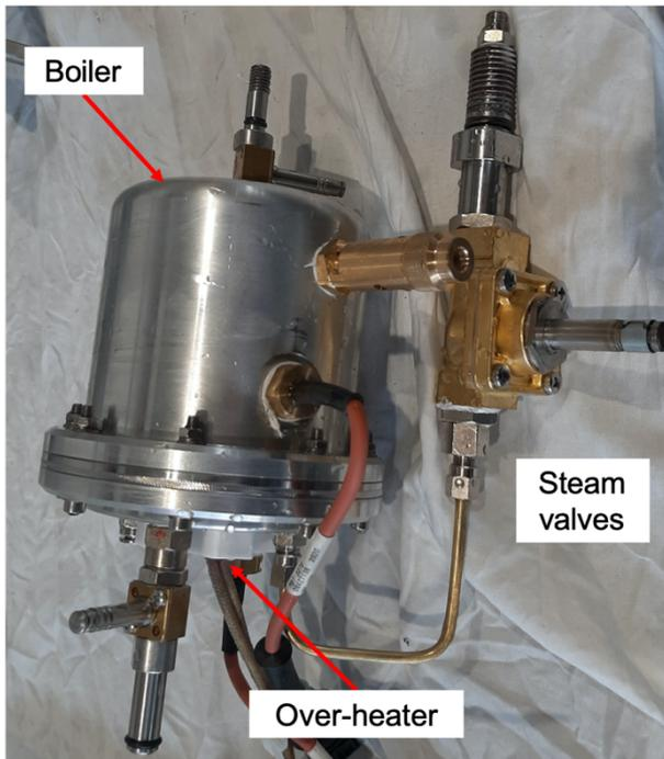
Figure 3: Boiler and over-heater prototype.
