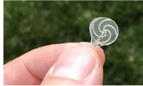
Fig. 3. A compliant, 10-mm diameter gas collector.
