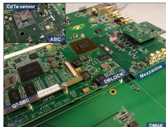
**Fig. 4.** Characterization setup to validate the digital integration concept with CdTe sensors.
