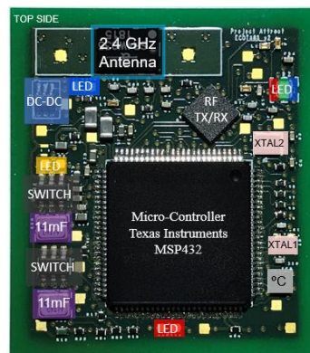
Fig. 2. Diagram of the different electronic components integrated in the final version of ECOTAGS prototype (left) and picture of the electronic assembly as-mounted on a PCB.
