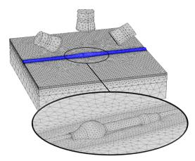
**Fig. 2.** 3D model of a hydrocephalus shunt (valve and catheters) under the skin and three transducers in a plane.
