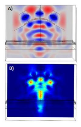
**Fig. 3.** Numerical results of a 3D computer simulation of the ultrasound field generated by the combination of three transducers emitting at 39 kHz in the middle plane. A) Acoustic pressure field (Pa). B) Acoustic power density (W/m<sup>2</sup>). Higher values are depicted in reddish tones.
