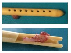
**Fig. 1.** Top: Explanted catheter (outer diameter of 2.7 mm) showing external deposit of about 2 mm in length. It also obstructs one of the draining holes of the tip. Bottom: Detail of the (sliced) tip showing accumulated debris (inside) that blocks CSF flow. Inner length of the deposit is about 10 mm.
