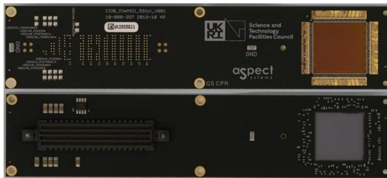
**Fig 1.** The high aspect ratio GP2M PCB. Front and back views of the same PCB. The sensor is mounted over the window seen bottom right. The board dimensions are  $185 \text{ mm} \times 40 \text{ mm}$ .
