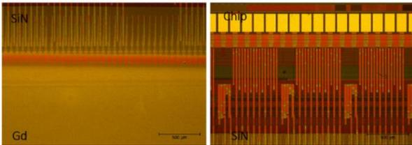
**Fig 2.** Close up of the SiN encapsulation. LEFT: Gadolinium covering the PImMS sensor pixels, with a larger area of SiN encapsulation also covering the metallic tracks. RIGHT: showing that the SiN encapsulation does not cover the bond pads, used to connect to the PCB. Scale bars measure 500  $\mu\text{m}$ .
