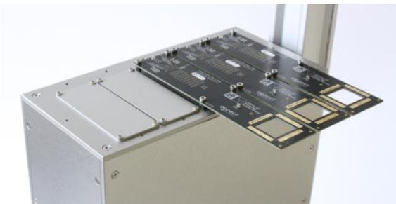
**Fig 3.** Three GP2M units populating a 5-slot chassis. Each camera is operated independently and can be placed in any slot or outside of the chassis entirely.
