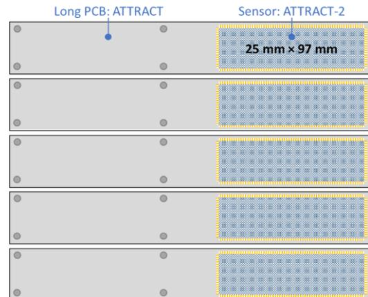
**Fig 4.** Camera system build using stitched sensors and the long-thin PCB developed within ATTRACT.
