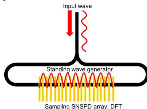
**Figure.1** Standing wave integrated Fourier transform. The device consists of a SiN waveguide formed in a loop to interfere the input signal with itself generating standing waves. The standing waves will be sampled an array of superconducting single photon detectors.
