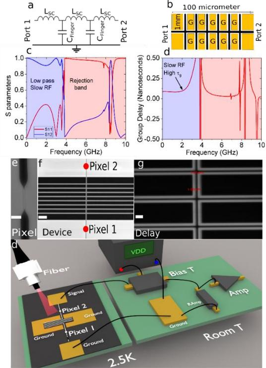
**Figure 3** (a) and (b) circuit diagram and schematic of the simulated structure. (c) and (d) S parameter and group delay of the simulated transmission line. SEM of one pixel (e), fabricated device (f), and delay element (g). (d) Schematic of the experimental setup
