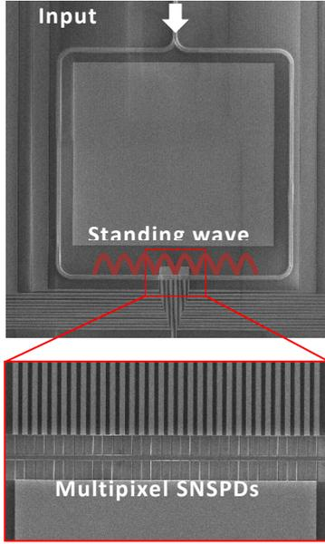
**Figure.2.** Fabricated spectrometer, consisting of a SiN interferometer with multi pixel single photon detectors.
