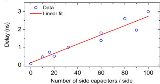
**Figure.4** Extracted delay for devices with different number of side-capacitors on each side, linearly fitted to a straight line. The slope of the linear fit is  $0.26\pm 0.03$  nanoseconds per 10 side-capacitors
