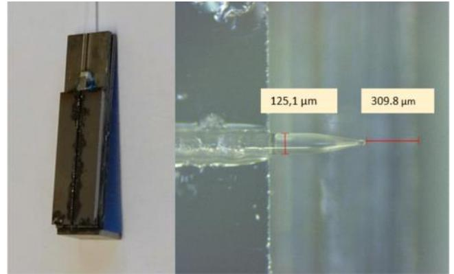
**Fig. 3.** Left: Image showing the assembled low temperature compatible optical connector that is mounted on top of the UTC-PD and attached to same carrier as PD. Right: Microscope image of the lensed fiber end, with measurements indicating the fiber diameter and offset distance to account for photodiode height. See Figure 4, detailing test complete test circuit.
