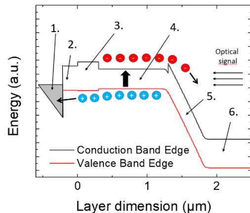
**Fig. 1.** Band diagram for novel UTC-PD design towards high performance low temperature PDs. Layers 1: p-metal, 2: transparent p-contact, 3: p- electron diffusion blocking layer, 4: p-absorption layer, 5: n- collector layer, 6: transparent contact layer. Interfacial layers, Fermi levels and carrier profiles omitted for simplicity.
