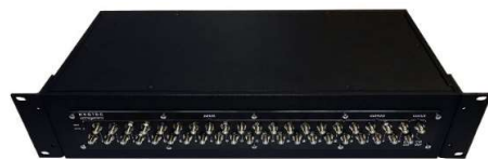
Fig. 1. The 19" rack mounted 32-channel NXGTDC prototype instrument.
