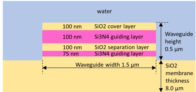
**Fig. 7:** Waveguide cross section.
