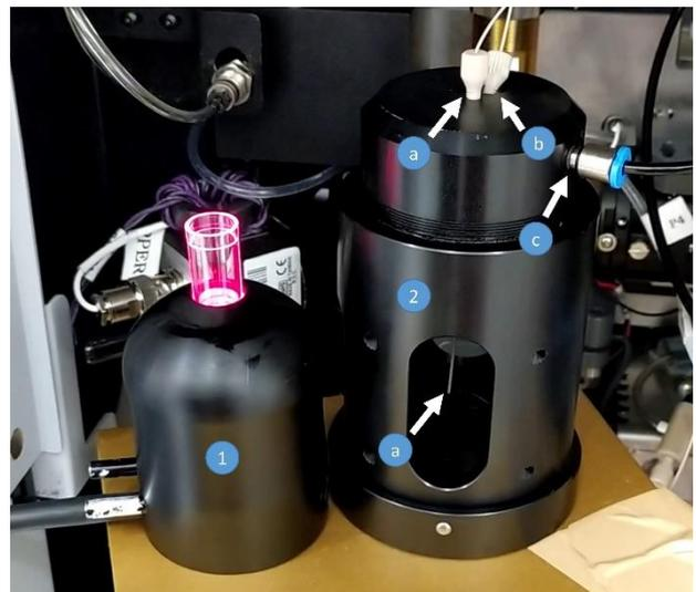
**Fig. 1.** Nr.1: pxONE illumination device with inserted sample tube; Nr.2: OptoCS prototype with connection tubes: (a) sample line (b) injection line (c) pressure line
