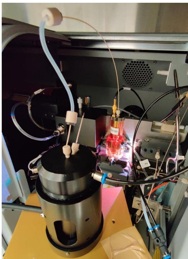
**Fig. 2.** The pxONE inserted in the OptoCS prototype and connected to a FACS Aria analysis chamber. The connection of the OptoCS prototype to the FACS Aria enables light stimulation and cell sorting at the same time.
