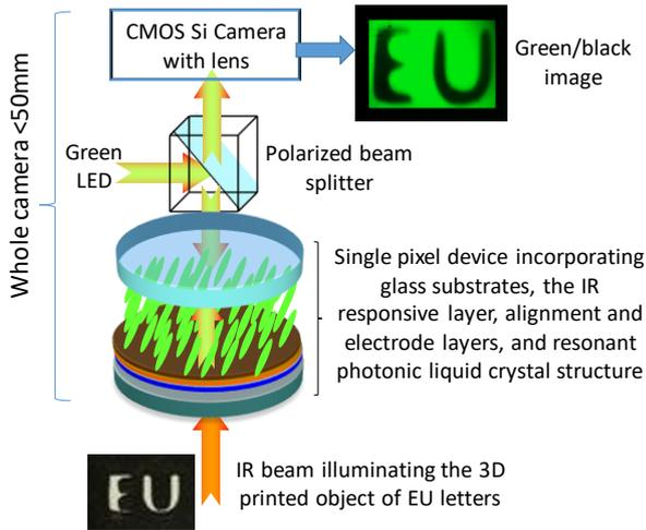
**Fig. 1.** Schematic of the thermal/IR single pixel imaging device integrated into Si camera. One example of IR illuminated object (EU letters) is shown as imaged with CMOS camera in green/black image in the 1<sup>st</sup> mode. The IR photosensor is a semiconductor sensitive to the SWIR range. Contrast is 70:1.
