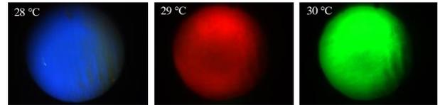
**Fig. 3.** Colour sequence variation of the blue phase LC as temperature increases, to explain the response to IR in Fig.2.
