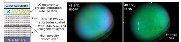
**Fig. 5.** Porous Si 1D photonic crystal/LC device (left) and the images read from the glass side using white light at IR OFF and ON. Due to heat diffusion in the Si substrate the slit image is not clear and the whole area changes colour quickly.
