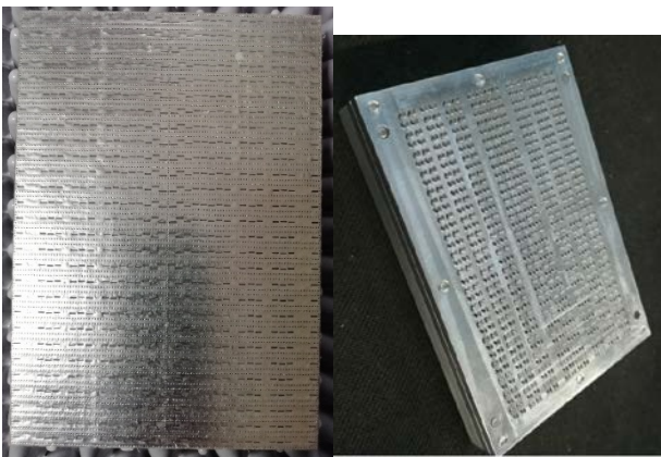
Fig. 3. (left) Prototype of the 77 GHz SIW radar antenna. (right) All-metal slotted waveguide array prototype with similar number of radiating slots built for benchmarking the SIW one.
