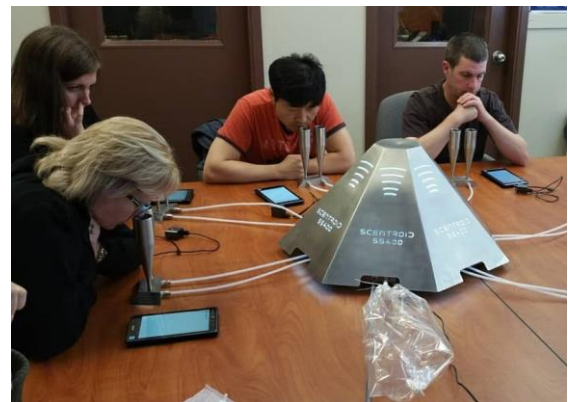
Fig. 3. Estimation of odour intensity by dynamic olfactometry. Reproduced with permission from Scentroid.
