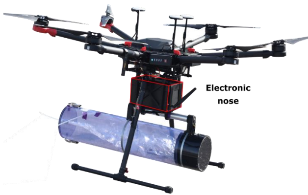
Fig. 2. Odour-sensitive drone carrying an electronic nose and an odour sampling device.
