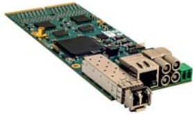
Fig. 5. A CAEN FERS unit (A5202) implementing the WeeROC CITIROC 1A ASIC.
